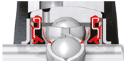
New Twin lip seal design for lubrication
